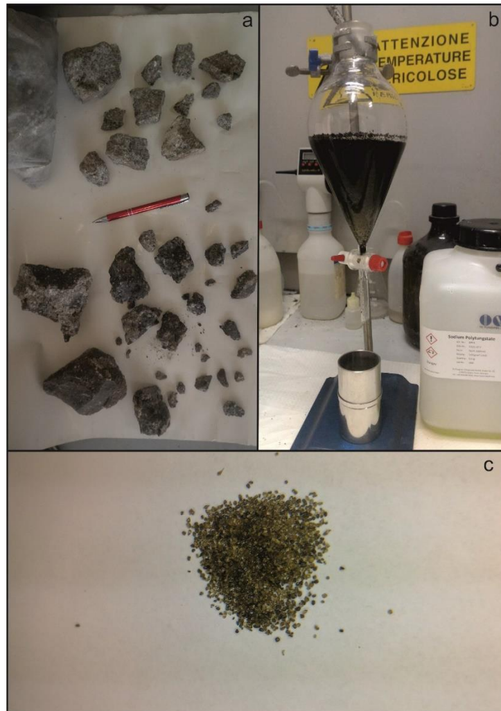
Figure 2.9 a) Mechanical separation of mafic inclusion in dacite rock from Ilopango dome. b) Separation of crystals with Sodium Polytungstate. c) Olivine crystals 0.5 mm.
