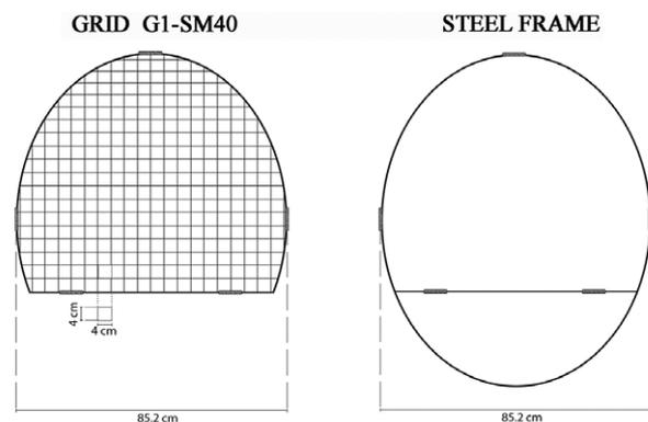
Fig. 2. – Designed sorting grid used in the present study: G1-SM40.
