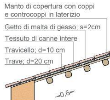
Fig. 6: Photo and digital return of the structural elements of a common roof of the masseria
