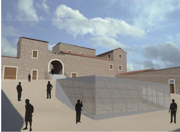
Fig. 14: Hypothesis of insertion of the solar greenhouse inside the courtyard at a lower level
