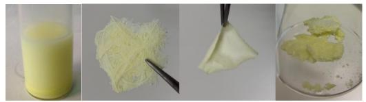
Figure. (From left to right) Nanoparticles dispersed in a solvent, Ce:YAG composites in glass wool, filter paper and cotton wool.
