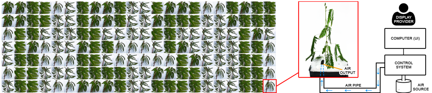
Figure 1. A conceptual plant-based display with multiple plants as pixels (plant-pixels or plantxels ) that close their leaves based on external stimuli (e.g. vibrations, touch, air flows, or electrical signals). The conceptual display is obtained by reproducing and arranging a single plantxel made of a Mimosa spegazzinii plant in its normal state (open leaves - darker green pixels) and when exposed to an air flow (closed leaves - revealing the white background). The plantxel is controlled by a prototype system developed to control the air flow from an air source to the plantxel as shown on the right.
