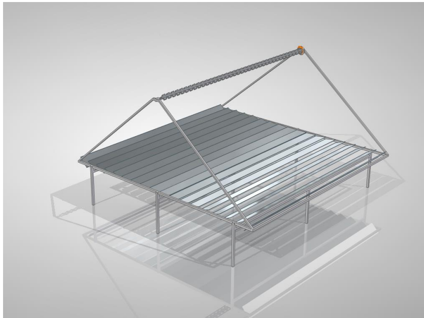
Figure 58. 3D rendering of a Fresnel type solar collector with second generation NAMTEC devices installed in a rotating array. Construction details and assembly are included on the relative patent request no. 102018000007710, deposited on 2018, July 31 st .
