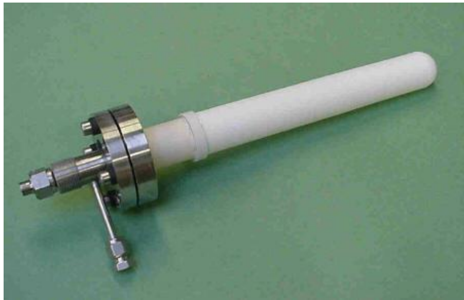
Figure 62. Beta '' -alumina ion conducting ceramic tube with ceramic-metal joining [56].
