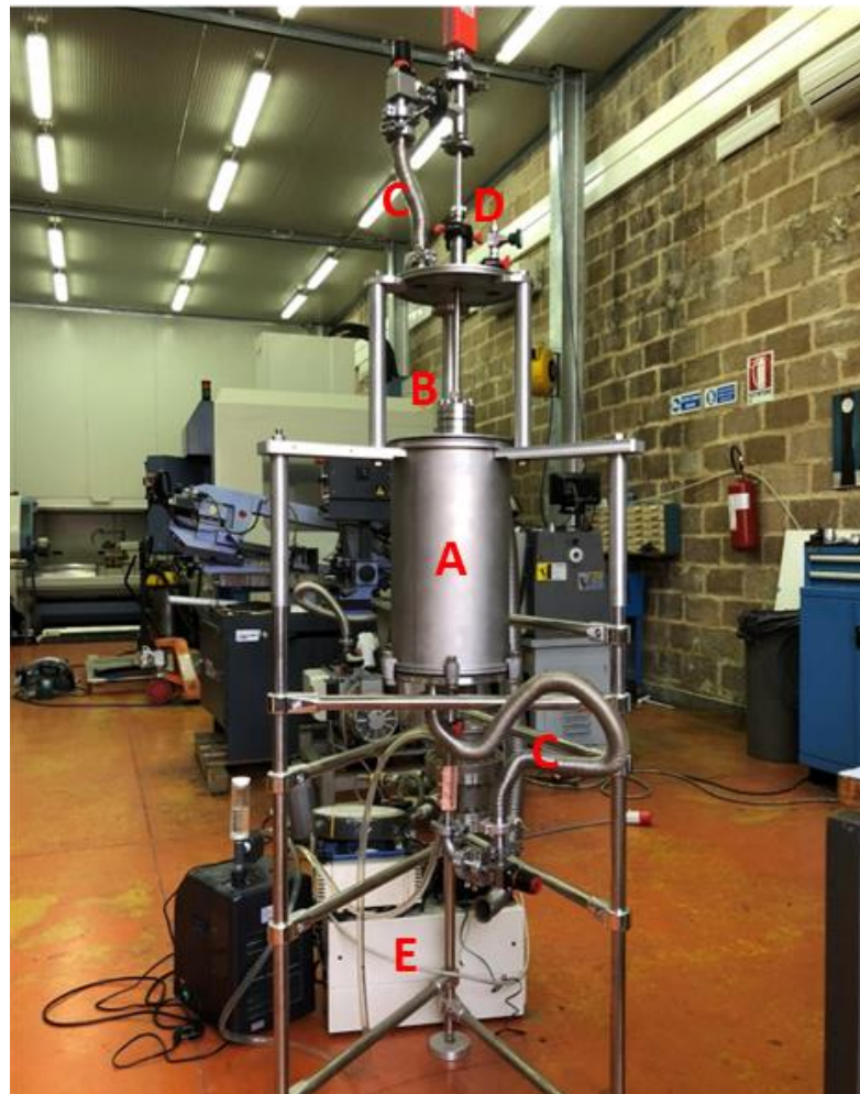
Figure 55. Proprietary developed experimental apparatus with indication of main items: (A) vacuum chamber; (B) experimental cell; (C) vacuum circuit; (D) feed-through system for power, control and signal connections; (E) vacuum pump.
