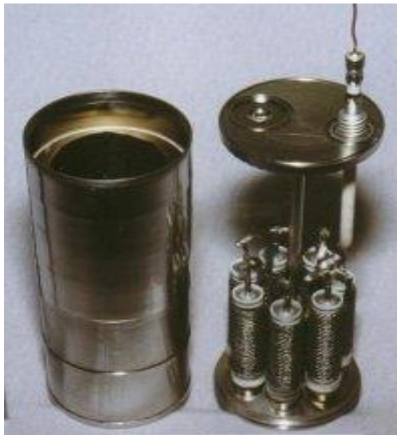
Figure 9. A particular configuration of an AMTEC converter with housing (left) removed [21].
