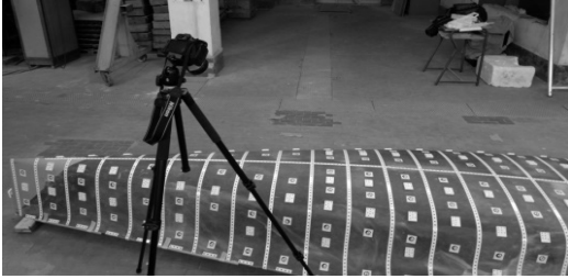
Fig. 4: Non-coded target applied on the hull surface
