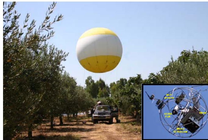
Figure 2. The tethered helium balloon during the launching phase. In the inset (lower right corner), there is an image of the proximity-sensing platform, which includes an MCA-II multispectral camera, an A320G thermal camera, a mini PC, and a wireless Wi-Fi omnidirectional antenna.
