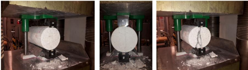
Figure 4.3. Characterization of the tensile strength of the concrete
