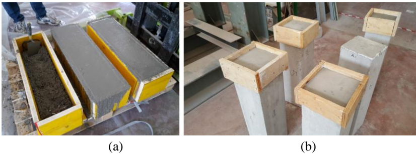
Figure 5.2. Casting of concrete (a); leveling of the specimen end-cross sections.
