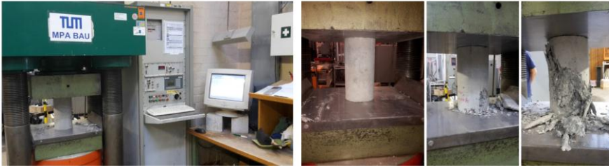
Figure 4.2. Characterization of the compressive strength and the elastic modulus of the concrete.
