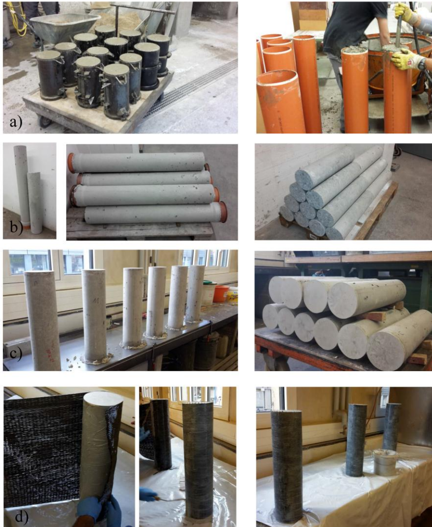
Figure 4.1. Preparation of the specimens: casting of the concrete (a); cutting the cylinders (b); leveling of the end cross-section (c); FRP wrapping (d).
