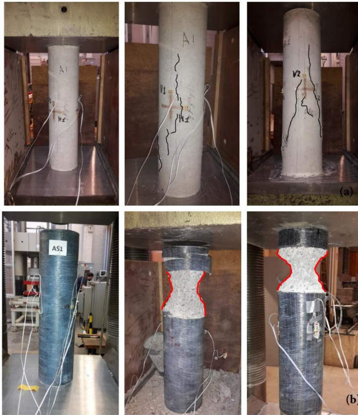
Figure 4.13. Unconfined and confined concrete specimens. Monotonic tests without preload.
