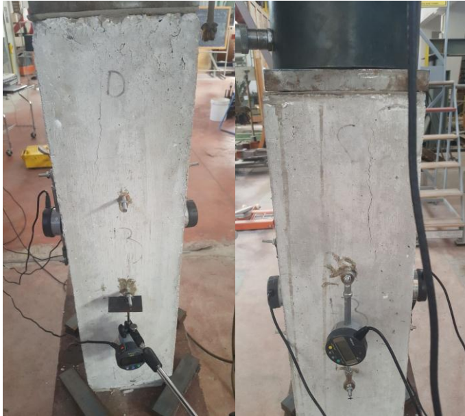
Figure 5.12. Evolution of cracking strain on specimen P80S2.
