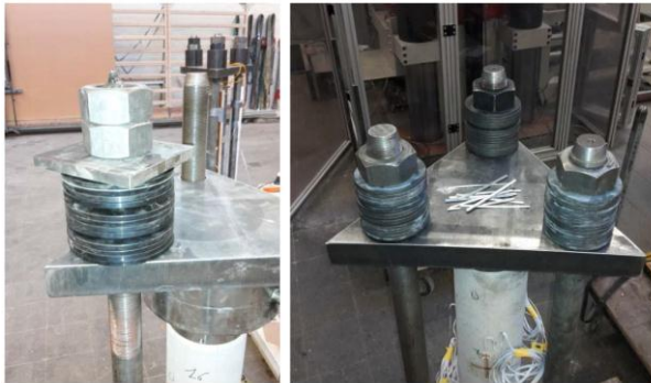
Figure 4.6. Disc springs used to keep constant the load on the specimens.
