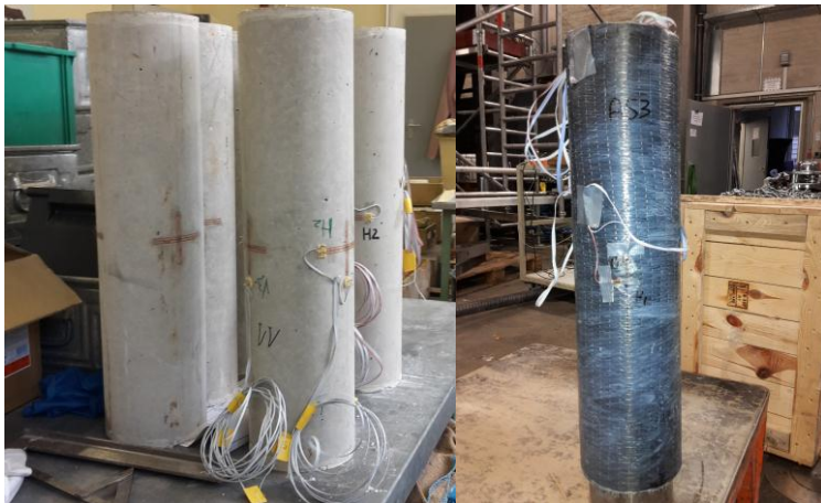
Figure 4.8. Application of strain gauges on the plain concrete and strengthened specimens.
