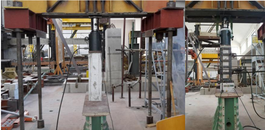
Figure 5.7. Preloading of a specimen and welding/application of the steel jackets after loading.
