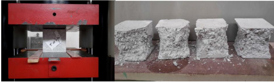
Figure 5.9. Compression tests on concrete cubes.
