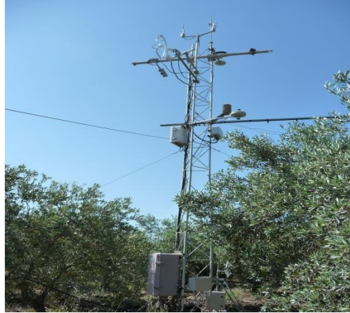
Figure. 3.18: Flux tower installed in the study area
