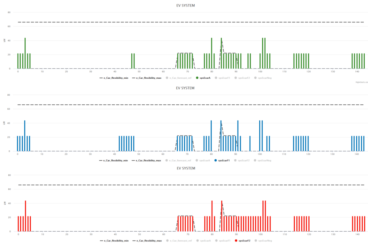
Figure 70 – The optimised solutions of the EV system energy unit provided by the DSS. Green bar: trade-off solution (A). Blue bar: solution providing the best fitness towards the first objective function (F1). Red bar: solution providing the best fitness towards the second objective function (F2).
