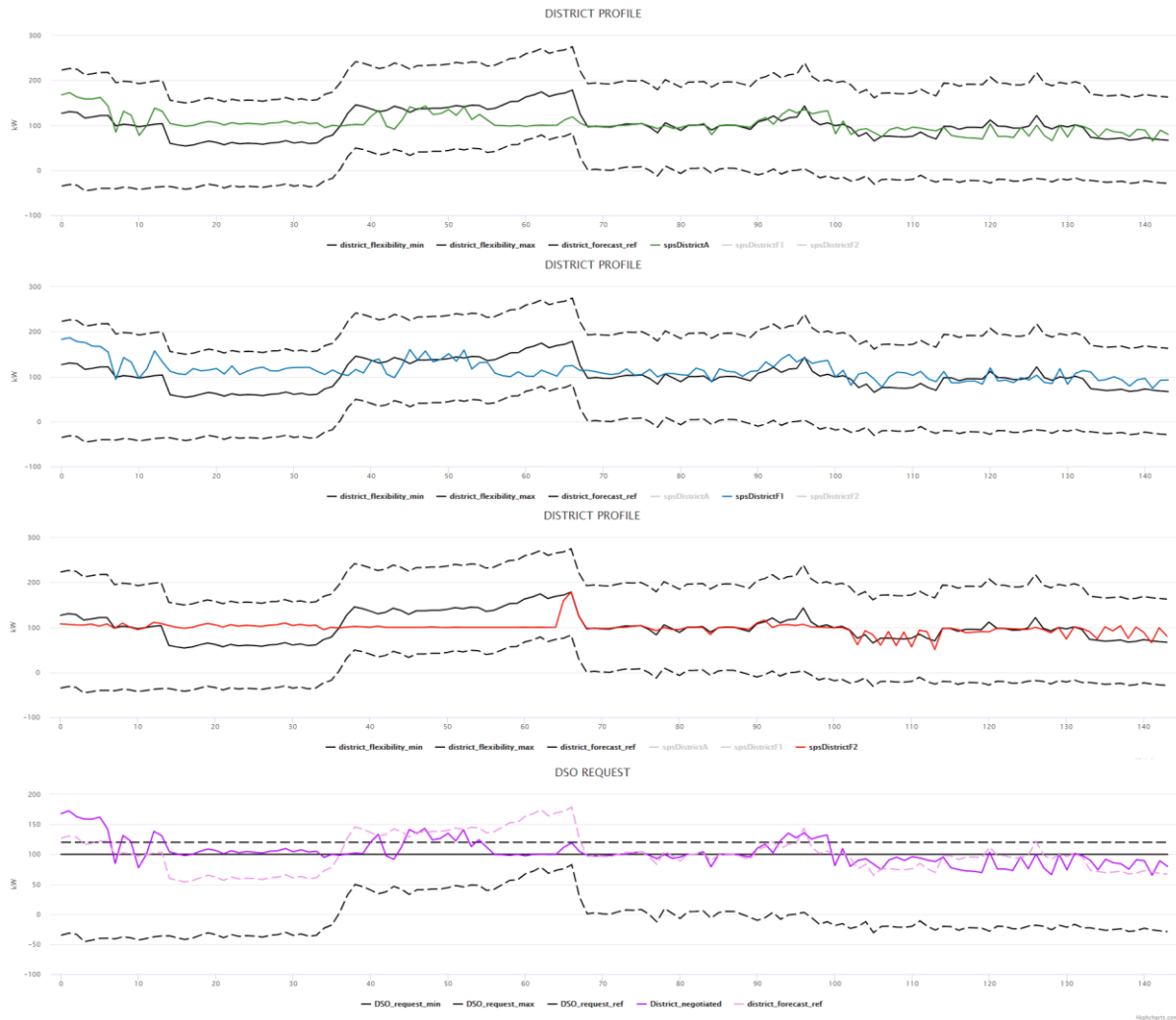
Figure 73 – The optimised power profiles of the district reported in comparison with the district forecast and the DSO power request. Green line: trade-off solution (A). Blue line: solution providing the best fitness towards the first objective function (F1). Red line: solution providing the best fitness towards the second objective function (F2). Purple line: negotiated solution.
