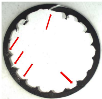
Figure 5-14. Photographic analysis of inner semicon defects
