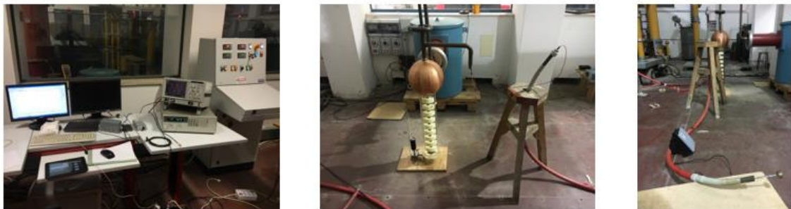
Figure 4-2. Measurement setup: arbitrary waveform generator, transformer and cable under test
