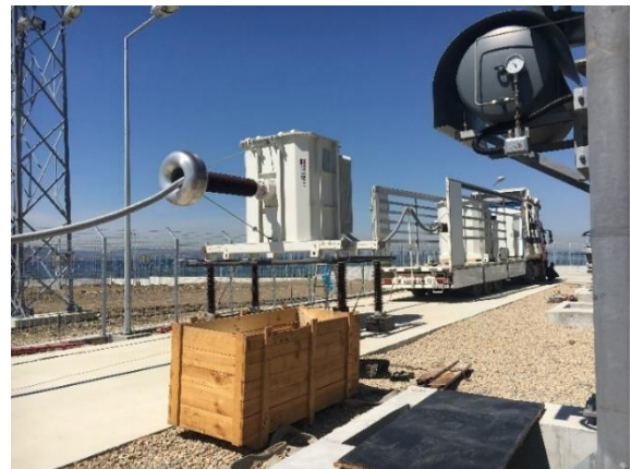
Figure 6-9. Resonant test system with reactors in series during the commissioning
