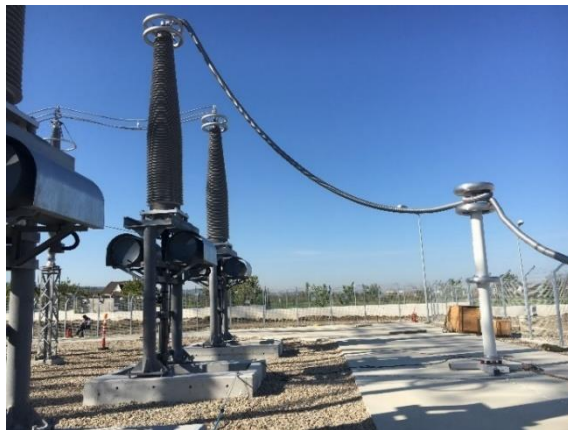
Figure 6-9. Resonant test system with reactors in series during the commissioning
