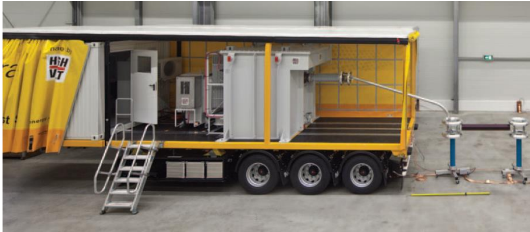
Figure 6-3. AC resonant test system for on-site testing of extruded HV cables
