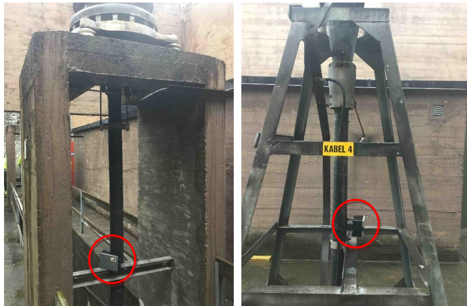
Figure 6-45. Pry-Cam portable placed on outdoor terminations
