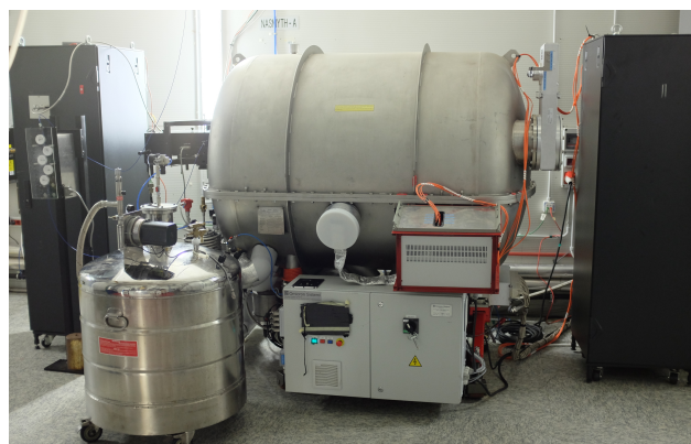
Figure 2.2: Picture of Giano dewar in the TNG Nasmyth-A. Figure taken from TNG webpage.
