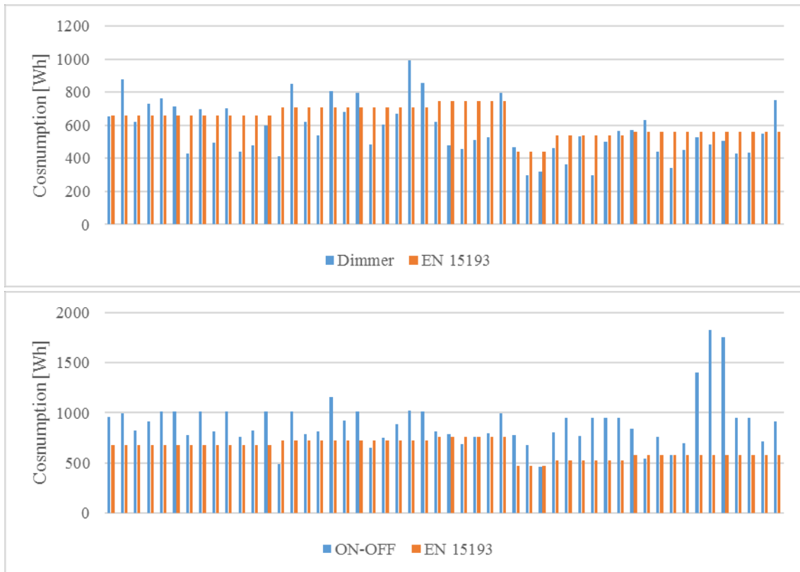
Figure 106. Comparison between consumption calculated using the comprehensive method and measured consumption for some scenarios in dimmer and ON-OFF cases
