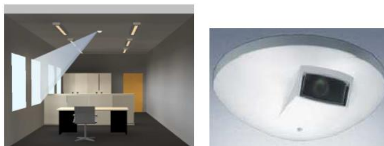
Figure 17. Open loop photosensor located indoor on the ceiling
