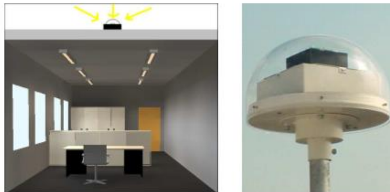
Figure 16. Openloop sensor located on the roof
