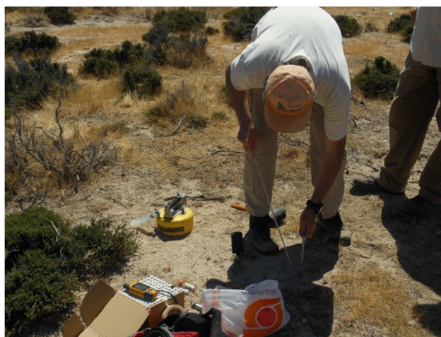
Fig. 7. 1- Soil gases sampling from the underground.
