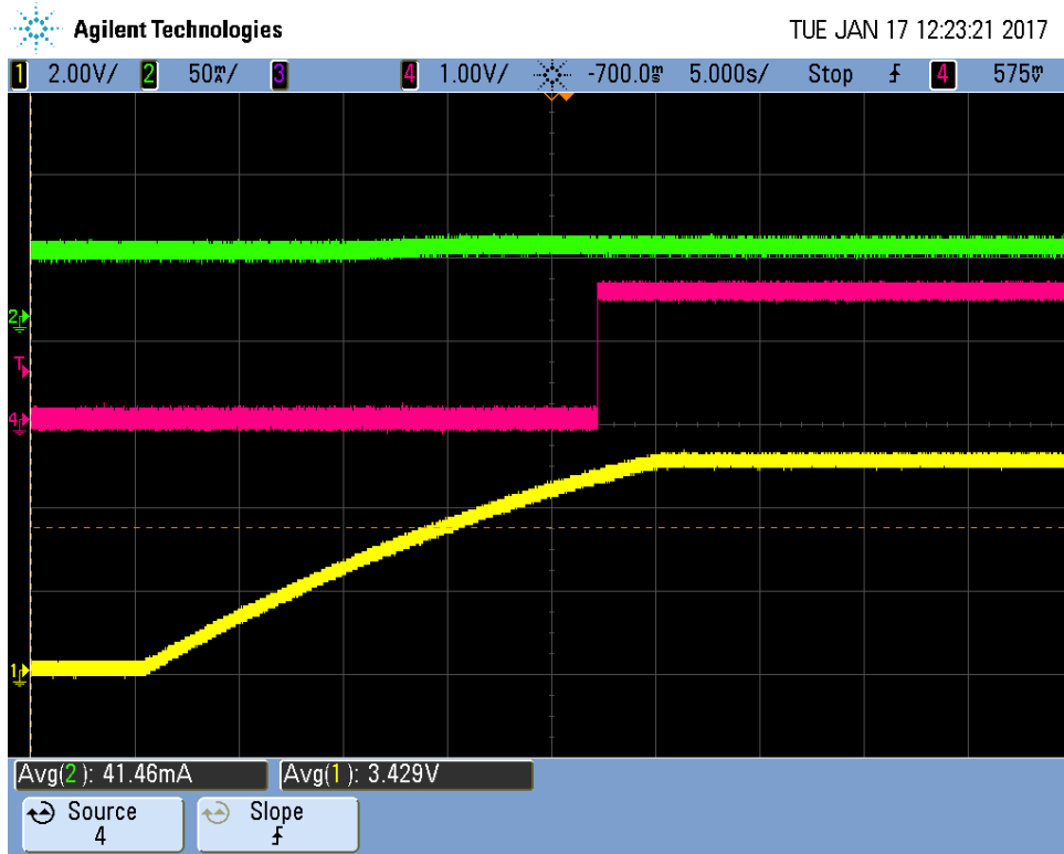
Figure 60: Time domain waveforms of input current I_{IN} (top), P_{GD} voltage (middle) and output voltage V_{STORE} (bottom)
