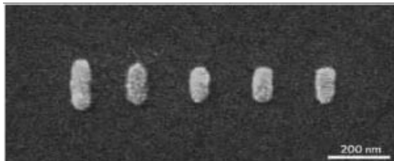
Figure 16: Yagi-Uda nanoantenna SEM image [27]
