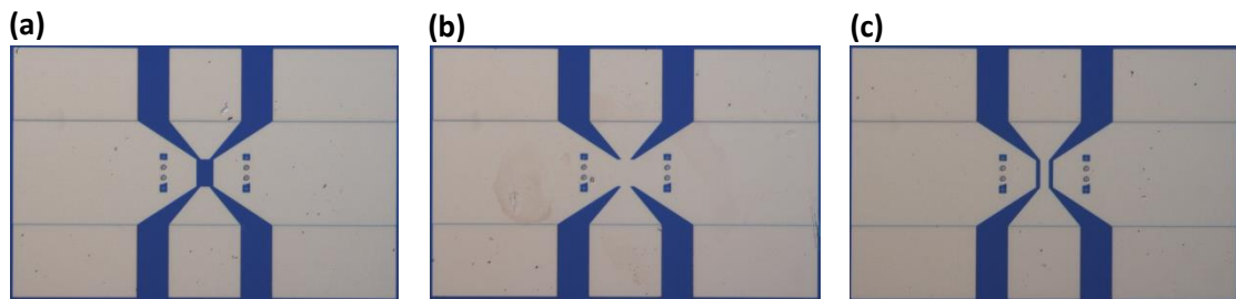
Fig. 3.12 – Micrographs of the test-devices fabricated to facilitate the de-embedding procedure, including: (a) “open”, (b) “short” and (c) “thru” structures.
