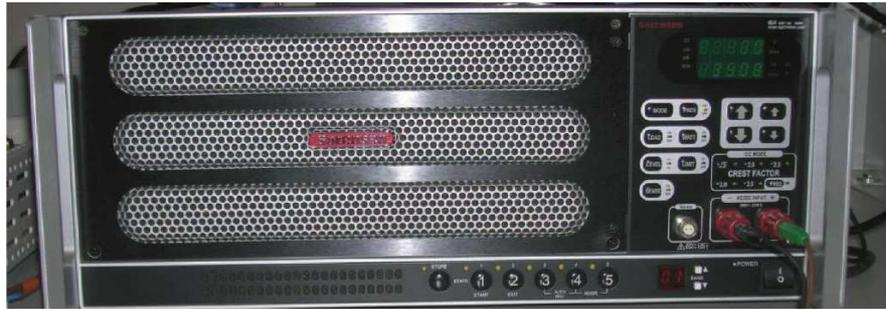
**Fig. 75** Carico elettronico Sorensen SLHACDC 500V 6A 1800W.
