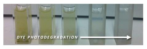
composition and electronic properties were investigated by XRD, Raman and photoelectron spectroscopies (XPS and UPS) while photocatalytic properties under both UV and visible light were studied by following the degradation kinetic of carminic acid by UV-Vis spectrophotometry.
