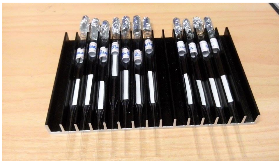
Figure 1. Glass Pasteur pipettes used to deliver stimulus volatiles to the antennae, each containing a piece of filter paper strip impregnated with a test compound or a mixture.
