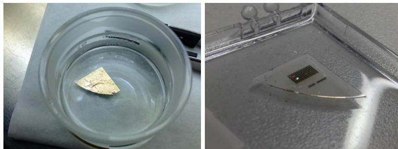
Fig. 3.15: lift off procedure
