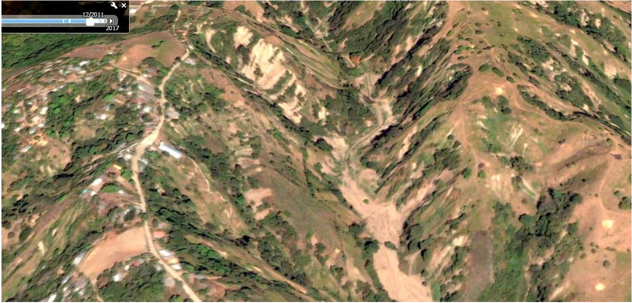
Fig. 5.11 – Effects of debris flood phenomena along the main stream valley, La Joya basin.
