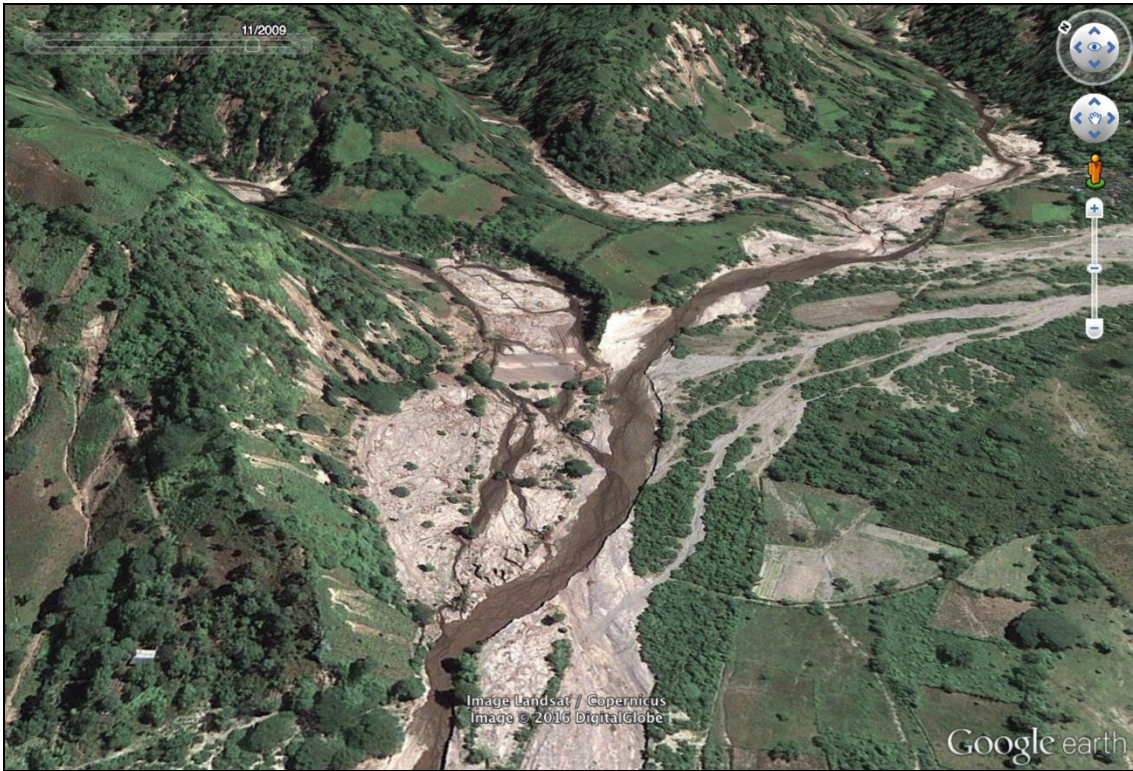
Fig. 5.2 – Effects of debris flood phenomena along the main stream valley.
