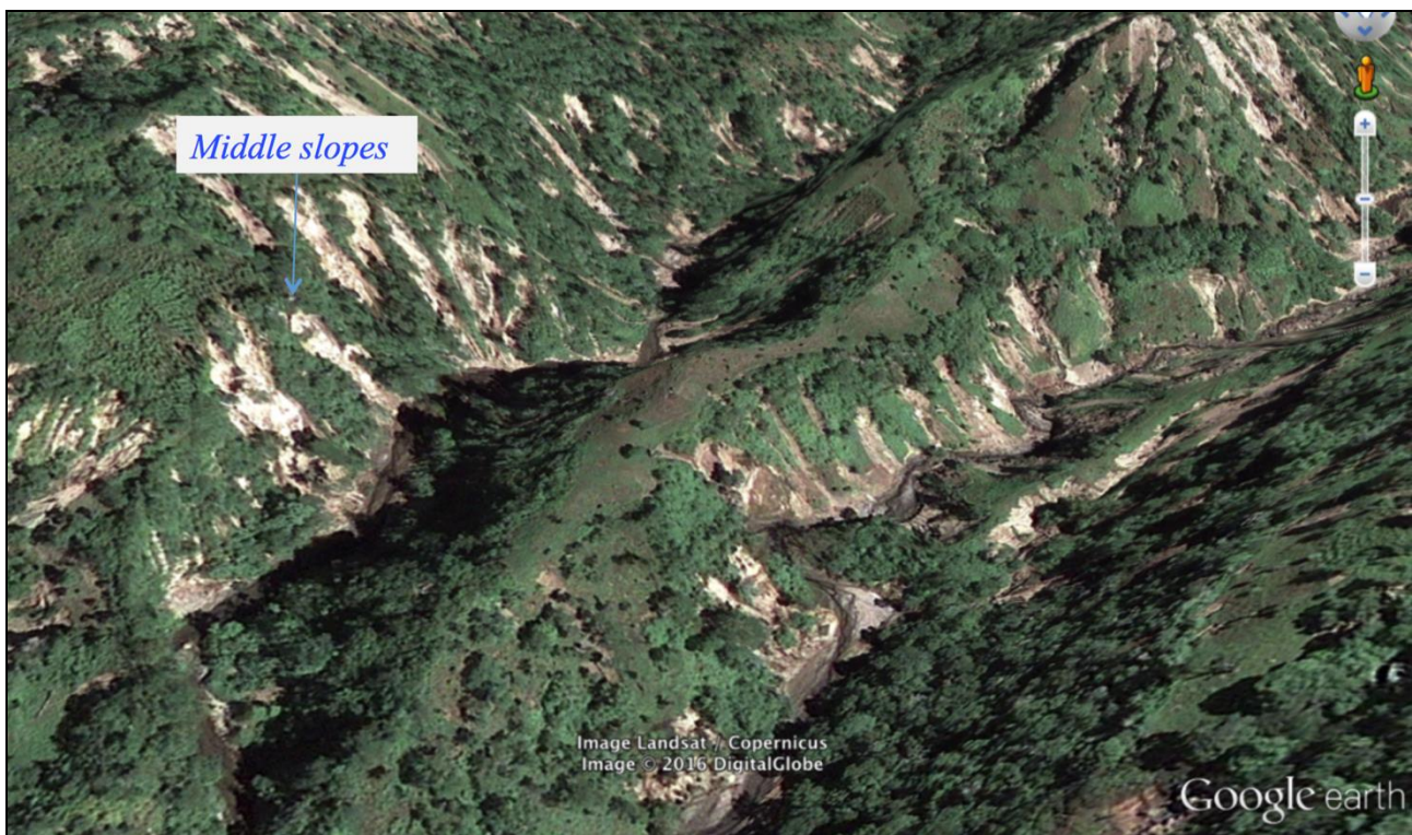
Fig. 5.3 – Examples of landslides activated from the middle part of the slopes in the Ilopango caldera.
