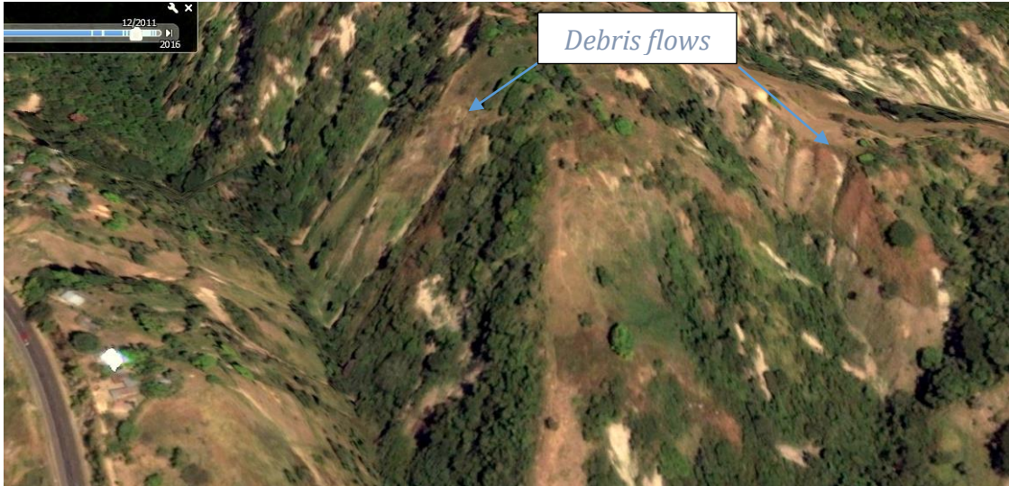
Fig. 5.13 – Examples of landslides activated as pure debris flows channelizing along the drainage network in the Coatepeque caldera.
