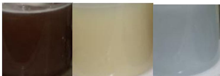
Figure 7.3. Lignin bleaching of Kraft Pulp during the APS process (Left: time zero; middle: after 2 h; right: after 12 h).
