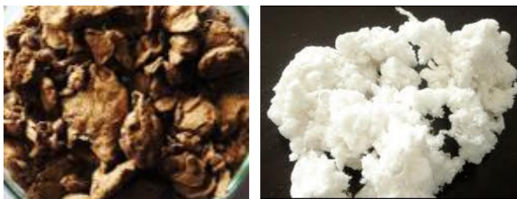
Figure 7.1. The raw materials used to obtain CNCs: Cotton linters (Left), Kraft pulp from softwood (Right).
