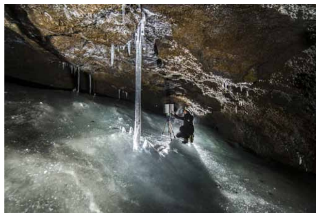
Figure 1. Scanning operations with the laser scanner inside the cave. The tripod was fixed with ice screws to scan on the ice floor (Photo: Alessio Romeo).
