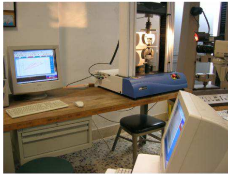
Figure A.2 Set-up for double cantilever beam test.
