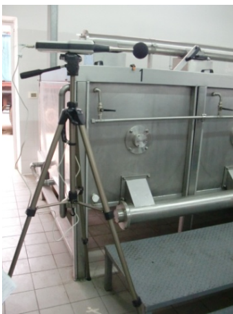
Figure 2: HD2110L integrating portable sound level meter by Delta OHM, Italy used in the tests. Figures and figure captions should be placed flush-left; two narrow figures may be placed side-by-side.
