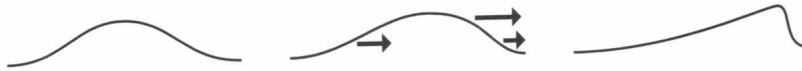
Figure 2.4: Formation of a shock wave by the steepening of a wave profile (Priest 2014).
