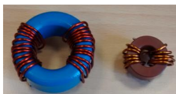
Figure III.16 - CM choke set up by using an N30 ferrite core (left) and a VITROPERM core (right).
