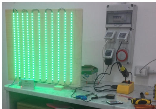
Figure 4.6 Led panels construction with ad-hoc welds.
