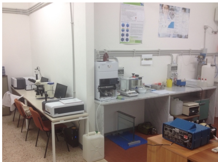
Figure 5.14. Internal lab view with the main equipment: HPLC (Agilent 1220 Infinity LC), spectrophotometer UV-Vis (Agilent Cary 60 UV-Vis), fluorescence spectrophotometer (Agilent Eclipse), precision balance (KERN ABJ-NM 80), optical and digital microscope (Optika B-800), FTIR (Agilent Cary 630 FTIR) and a Hydraulic Press (Pike CrushIR).
