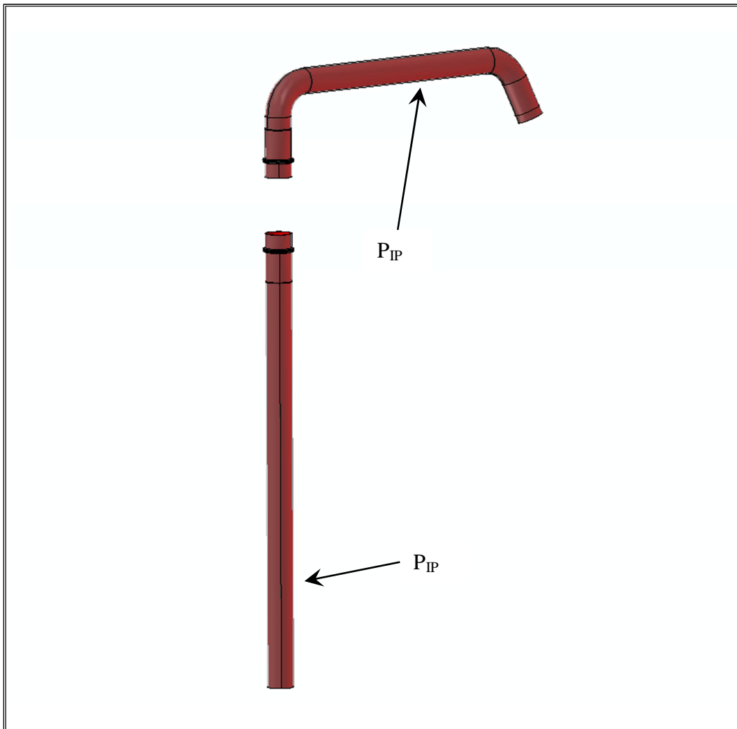
Figure 4-22. Lithium inlet pipe internal surfaces.
