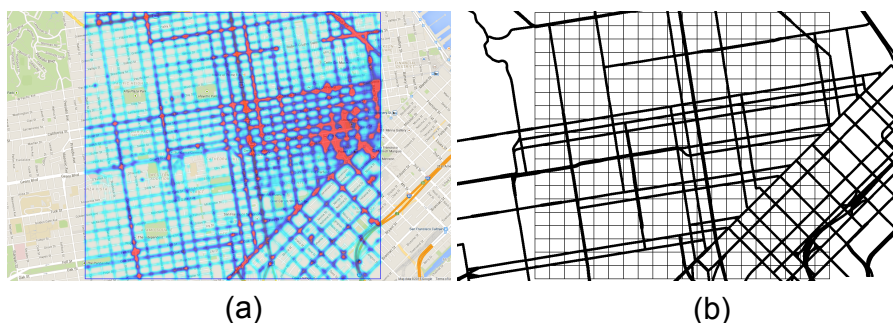
Figure 5.5: (a) Heatmap of mobility traces vs. (b) Arterial roads.
