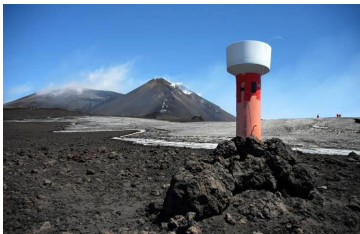
Figure 8: Collectors installed for the bulk deposition sampling.
