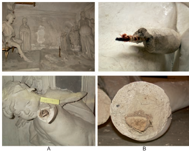
Figure 3. The wooden reinforcement and the succession of different layers of stucco in damaged statues from the S. Mercurio Oratory (A) and the Stigmata Monastery (B). Technical file for electronic storage of the results of the mineralogical petrographic analysis.
