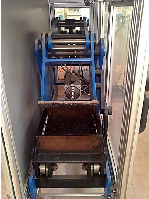
Fig. A.17 The compaction of slabs for WTT by roller compactor (Palermo)
