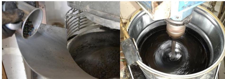
Fig. 2.5 Addition of the additive: in the mixing (DRY process, on the left), into the bitumen (WET process, on the right)
