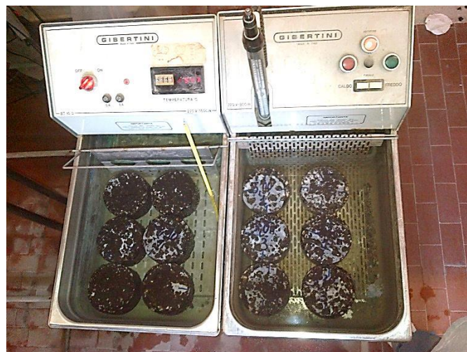
Fig. A.13 Thermostatic water bath before the Marshall Stability test (Palermo)
