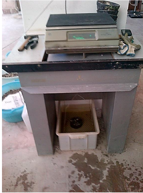
Fig. A.15 Hydrostatic balance (Palermo)
