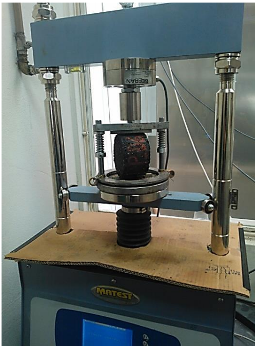
Fig. A.8 The ITS test on specimens subjected to the water sensitivity test (Guimarães)
