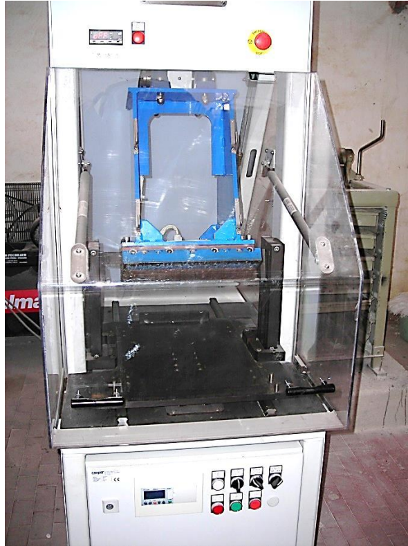
Fig. A.19 The roller compactor for slabs (Palermo)
