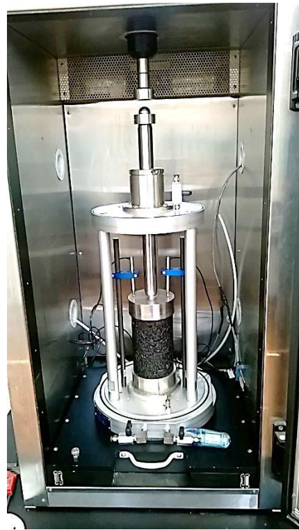
Fig. A.25 Modulus test by means of a triaxial cell (Palermo)
