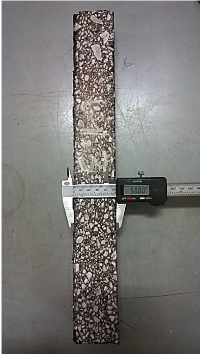
Fig. A.21 Specimen subjected to the four-point bending test (Palermo)
