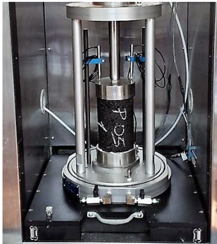
Fig. A.24 Specimen subjected to the modulus test (Palermo)
