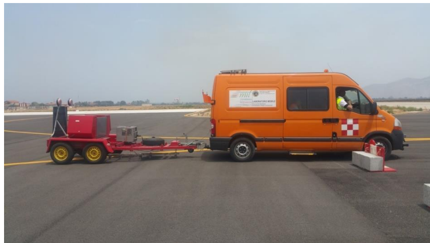
Fig. 4.12 Dynatest testing equipment
