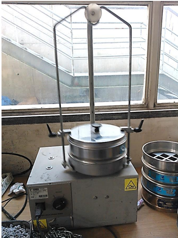
Fig. A.1 Sieving machine (Guimarães)
