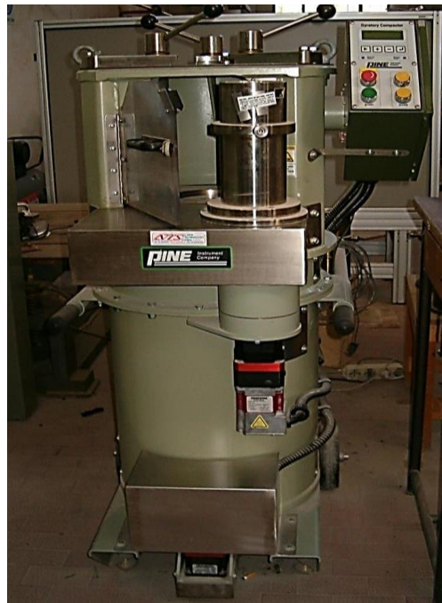
Fig. A.16 Gyrotory compactor (Palermo)
