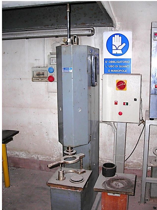
Fig. A.12 Automatic impact Marshall compactor (Palermo)
