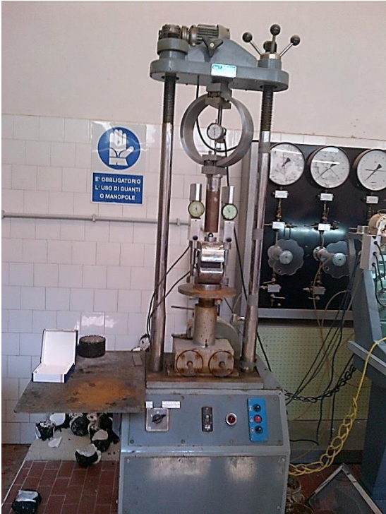
Fig. A.14 The Marshall Stability test (Palermo)
