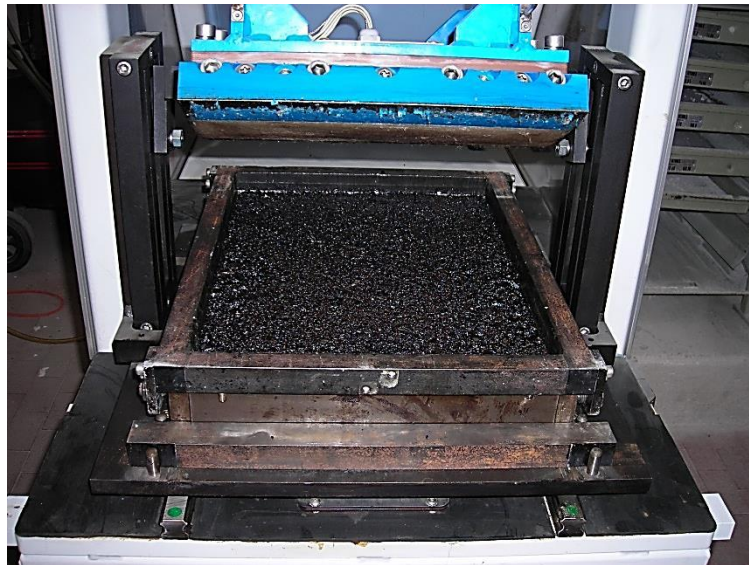
Fig. A.20 Slab after compaction (Palermo)
