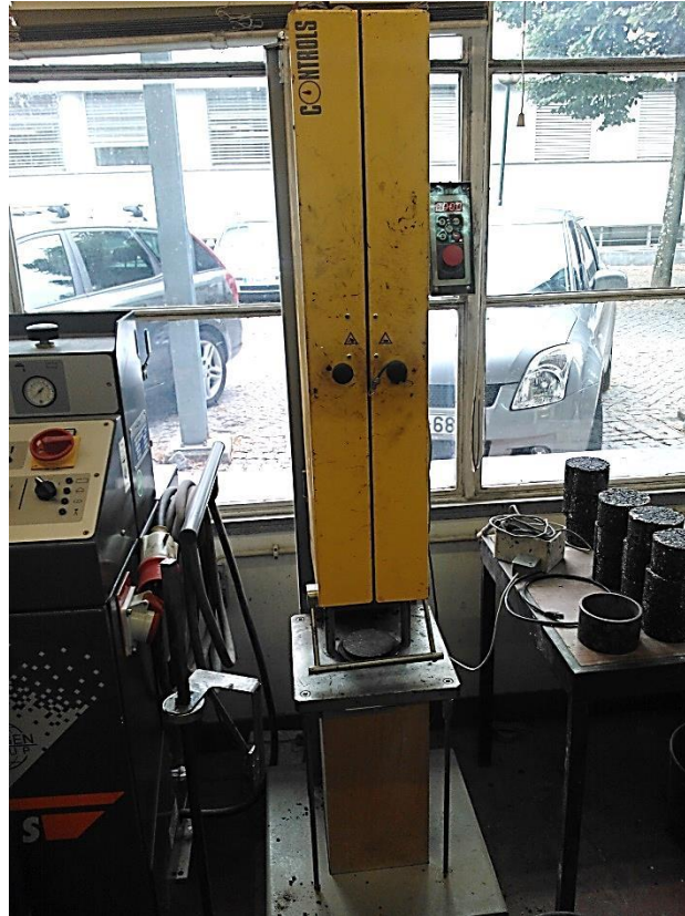
Fig. A.5 Automatic impact Marshall compactor (Guimarães)
