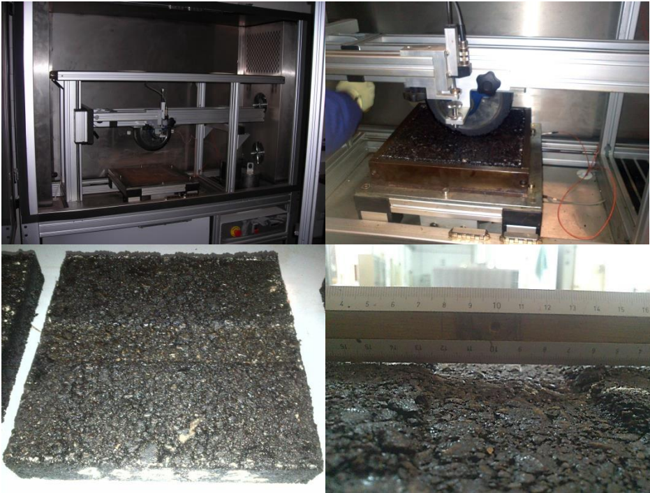
Fig. A.18 The stages of a wheel tracker test (Palermo)
