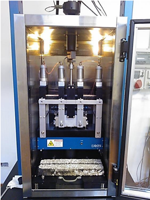
Fig. A.22 The four-point bending test device (Palermo)
