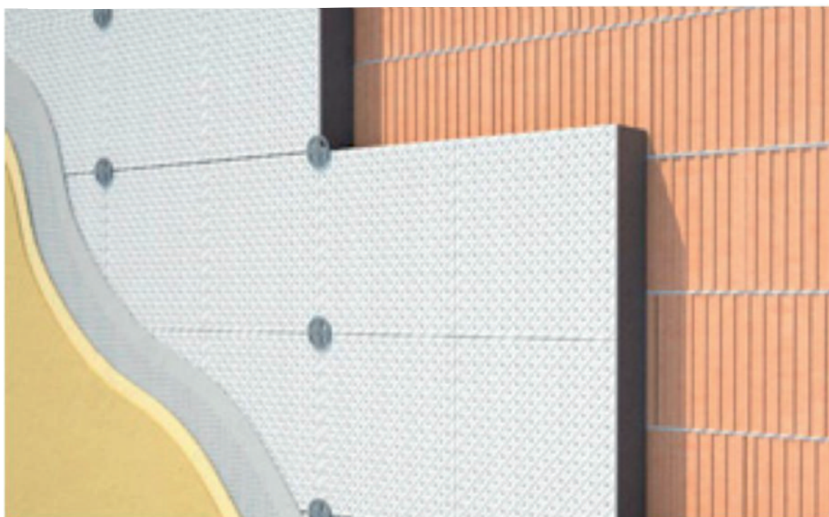
Figure 7: Scheme of application of the insulating panel from the inner face of the wall.
