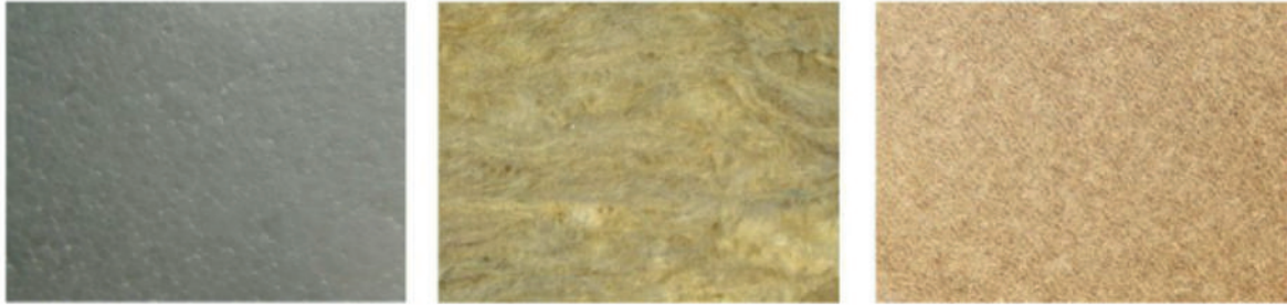
Figure 1: Materials commonly used for the insulation of the opaque envelope. From left to right: polystyrene foam (synthetic), rock wool (mineral) and wood wool (natural).
