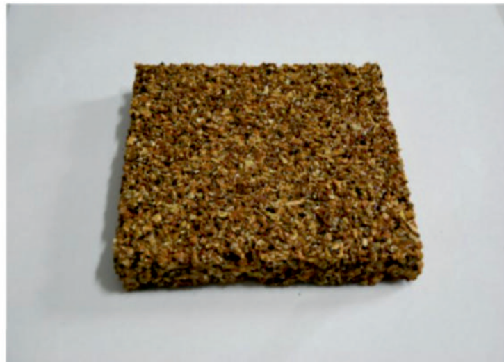
Figure 5: Final product: the Opuntia ficus-indica rigid panel
