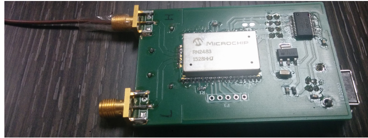
Figure 3.11: The LoRa-to-UART (and USB) interface used for testing the coverage.
