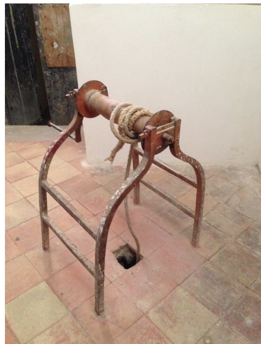
Figure 17. The monkey winch for lowering the central square plate of the Mathematical Table. On its back, it is possible to catch sight of the underground passage joining the cuisine to the butler's pantry just underneath the dining room.
