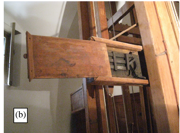
Figure 19. (a) Coloured strings used to order the desired dish or beverage. (b) Tinkling device operated by the string command.
