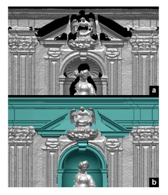
Figure 10. Area of the tympanum: a) triangulated surface from laser scanning data, b) integration with CAD models
