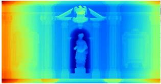
Figure 11. DSM used in orthorectification process
