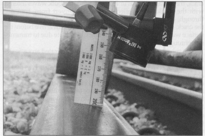
Figure 4 — Air coupled transducer configuration for vertical split head testing.
