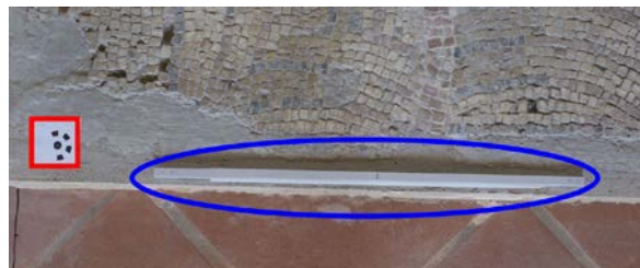
Fig. 4. Example of coded target (in red) and scale bar (in blue).
