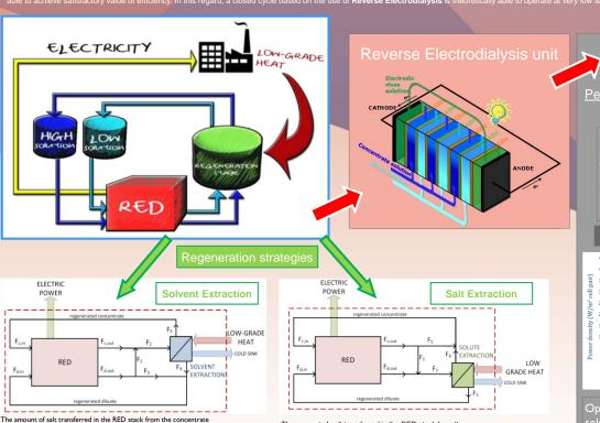
The amount of salt transferred in the RED stack from the concentrate solution to the diluted one is rebalanced by the preliminary addition of stream  $F_1$  to  $F_2$ . Then stream  $F_2$  is subjected to the necessary solvent excess extraction which results into two exiting streams, i.e. one solute rich  $F_2$  and one solute free  $F_{e\mu}$  which regenerate the two input streams necessary for RED system operation.
