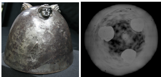
Fig. 5. X-Ray acquisition on Mastòs (NI 9): upper-lower projection
