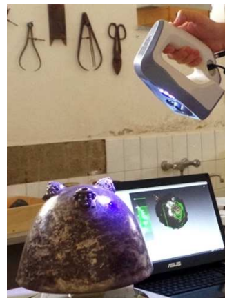
Fig. 2. Acquisition phase via 3D scanning of a piece of the collection.
