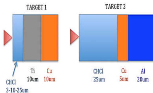
Figure 8-3 two main multi-layered targets made by a variable CHCl layer and thin layers of Ti, Al or Cu.
