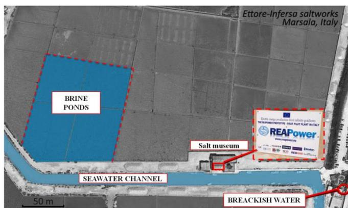
**Figure 4.1** Satellite image of the REAPower plant installation site (*Ettore-Infersa* saltworks, Marsala, Italy). Three different solutions are available for power production by RED: saturated brine from ponds, seawater from an open channel and brackish water.
