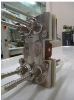
**Figure 3.35** Photo of stack assembled with 10 cell pairs and characterized by electrodes with a geometric area of 28 cm<sup>2</sup>.
