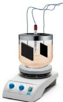
**Figure 9.4** Undivided cell maintained under magnetic stirrer and on constant temperature of  $30^{\circ}\text{C}$  to pre-acclimate the anode and to form the bio-anode with a film of *Shewanella putrefaciens*.
