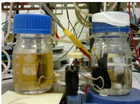
**Figure 6.4** Bicompart MFC with “H-configuration”.
