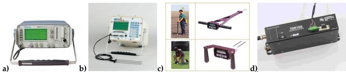
Figura 3.8 - Apparecchi TDR: a) Tektronix 1502C (Tektronix Inc.), TRASE System I (Soil Moisture equipment Corp.), c) Field Scout TDR300 (Spectrum Technologies, Inc), d) TDR100 (Campbell Scientific Inc.)
