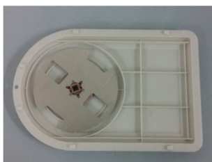
Figure 4.7 The metal turning disk and its plastic protection cover removed from the Fimar oven
