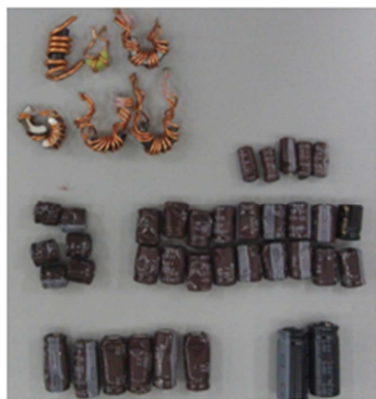
Figure 4.27 Capacitive and inductive components and others removed from the MB
