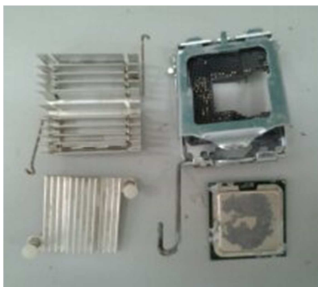
Figure 4.26 Bulky components removed from the MB
