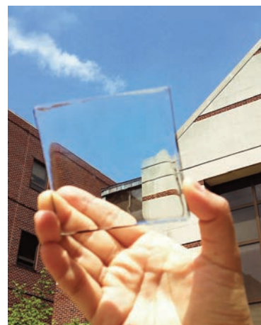
Photo 45 - Prototype of transparent solar cell according to Ubiquitous Energy technology
