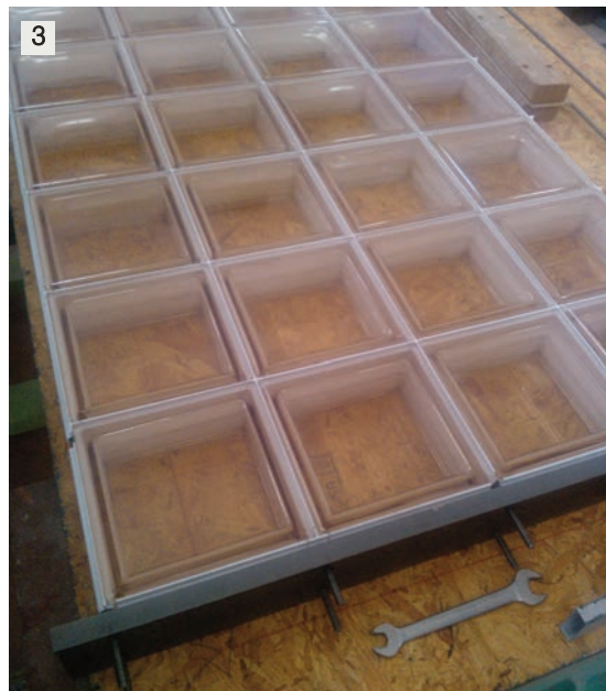
Photo 5 - Photos illustrating different phases of the assembly process of a prototype of a precast, dry-assembled panel made of "standard" glass blocks: 1) positioning of the first plastic profiles; 2) positioning of the first rows of glass blocks; 3) completion of the panel assembly, immediately before the prestressing of the bars; 4) vertical positioning of the prestressed panel;
