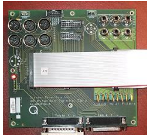
Fig. A.3 - Extended terminal board.
