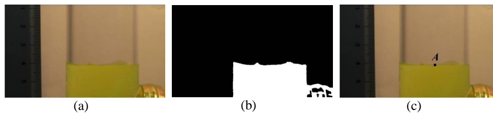
Fig. 3.17 – Image processing; (a) extracted frame from the video; (b) binary image; (c) image with the determined pixel position (black point on the water interface).
