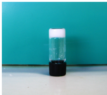
Figure 23: opaque gel formed by [p-C_{10im}][Br]_2 (5%, w/w) in the presence of two equivalents of \beta -CD.
