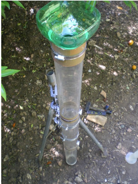
Figure 1. Device used to ensure flow verticality and to prevent wind effects during the runs with a height of water application of 1.5 m
