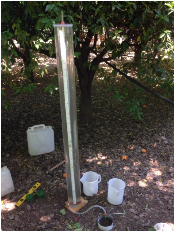
Figure 1. Mariotte bottle used for the long duration infiltration runs
